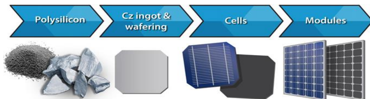
Figure 1: Solar (c-Si) PV Manufacturing Value Chain NREL, 2012
